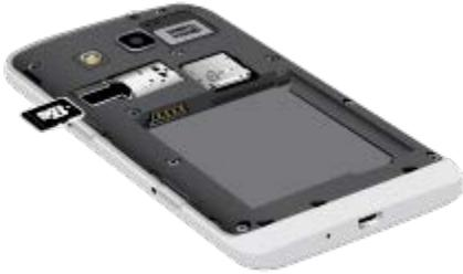
1. Using the slot provided, gently lift the cover off the phone.
