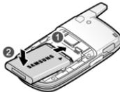
3. With the battery in position on the phone, place the cover back on the handset and slide it in until it clicks.
