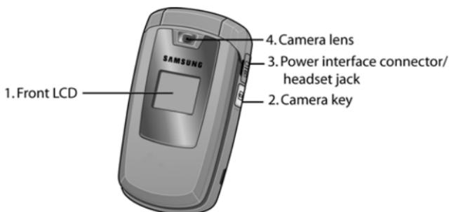
1. **Front LCD:** Your phone has an LCD display on the front that indicates when you have an incoming call or message. It also displays date,
