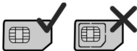
Insert the SIM card in the card slot. Be sure that the SIM card is facing in the right direction, as shown in figure 2, and then slide the SIM card into the slot.
