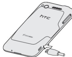
As the battery is being charged, the notification LED shows a solid amber light. The light turns to solid green when the phone is fully charged.
