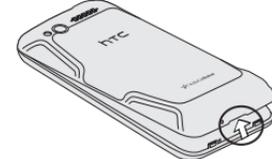
2. Take the battery out and remove the thin film that's wrapped around it.
