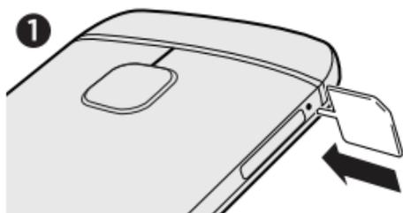
1. With the phone facing **down**, insert the tip of the tray eject tool that came with your phone (or a small bent paperclip) into the hole next to the nano SIM card tray that's on the left side of the phone.
