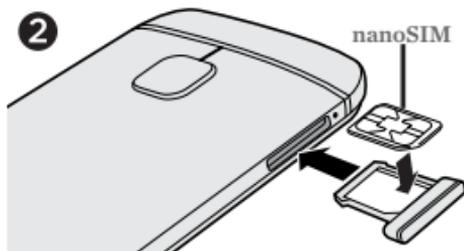
2. Place your nano SIM card into the tray, with the gold contacts facing **up** and cut-off corner facing **out**.
