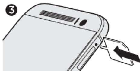
3. Flip the phone over and use the same tray eject tool to eject the microSD™ card tray that's on the right side of the phone. Pull the tray out.
