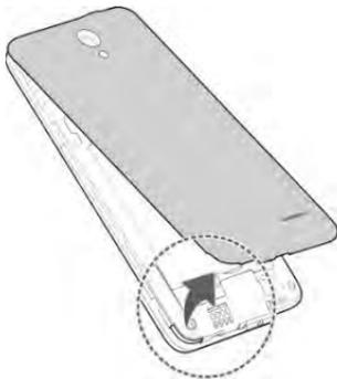
2. Hold the Nano-SIM card with the cut corner oriented as shown and slip them into the card holder.
