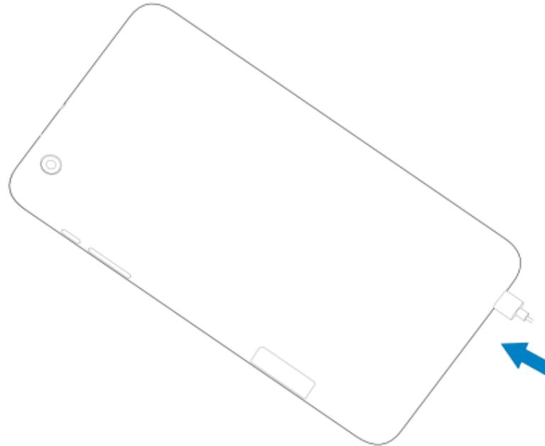
2. Connect the charger to a standard AC power outlet. If the device is on, you'll see a charging icon, such as
