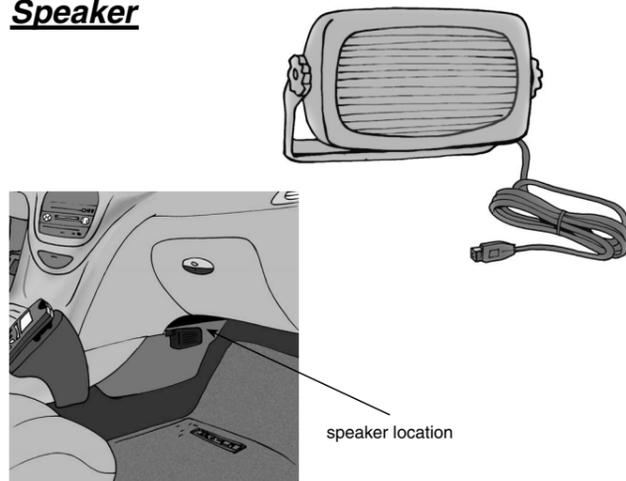
Install the speaker on the side of the central console, ideally alongside the legs of the passenger sitting beside the driver, as far as possible from the microphone.
