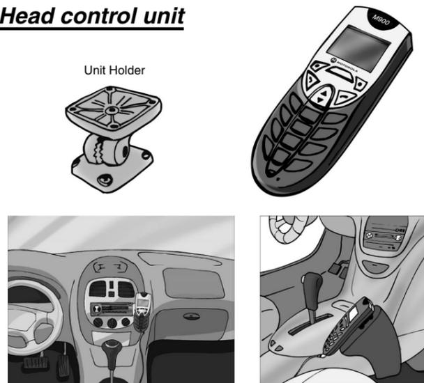
When installing the fixed mobile car phone avoid positioning the head control unit where it may disrupt the proper operation of the vehicle and/or its components, such as car stereo, air bags, cubbyhole, glove compartment, ashtray, lighter, gear stick, hand brake, etc....
