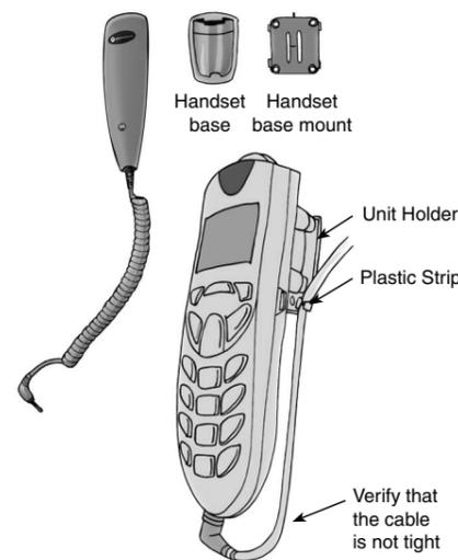
Mount the privacy handset using the plastic base and connect the handset jack to the socket at the bottom of the main control unit.
