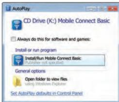
Select **Install/Run Mobile Connect Basic**. If this prompt does not appear, you can manually install the software by selecting **Start > Run > d:\setup.exe**
